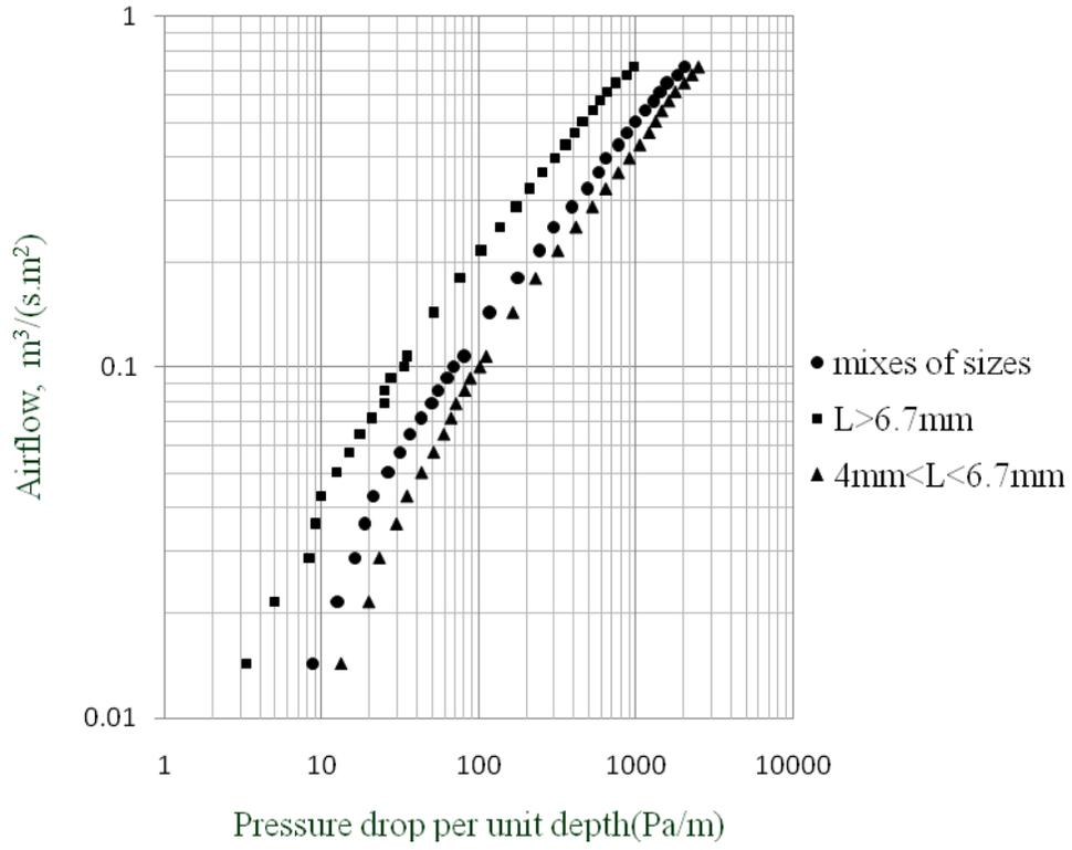
**Fig. 4- Resistance of white wood pellets with different sizes to air flow**
