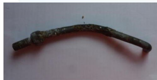
Shovels removed prior to the blast event, and tramp metal found after the incident believed to be the cause
